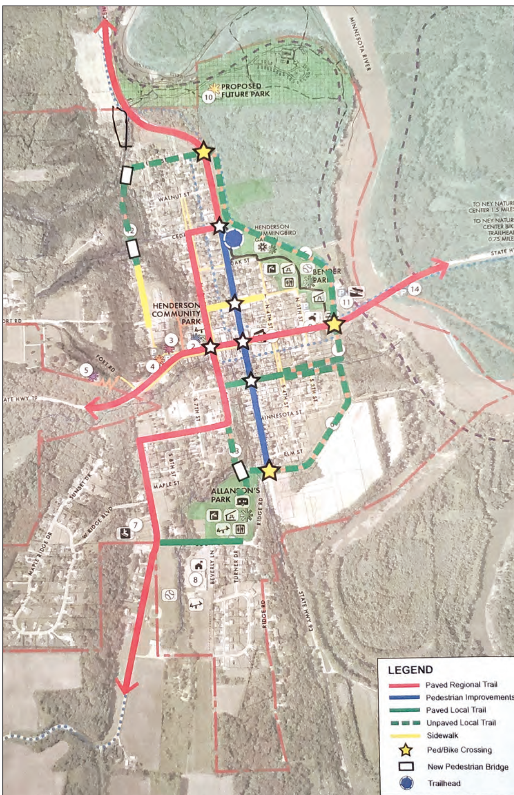
The above graphic shows the proposed Henderson trail system, complete with pedestrian/bike crossings (stars). The red line shows the paved regional trail, green is paved local trails, and blue is pedestrian improvements.
