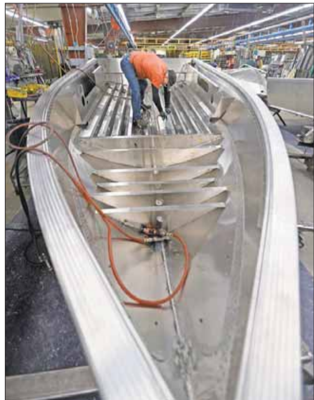
Boats are riveted at the Lund Boat Company in New York Mills, Minnesota.
