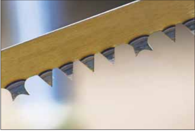
Above: Tom Segal, left, and Grant Segal hold Tuff Camp Saws on Friday at Spring Creek Manufacturing in Mountain Iron. Below: Every fifth tooth on the blade of a Tuff Camp Saw is called a “raker.”
