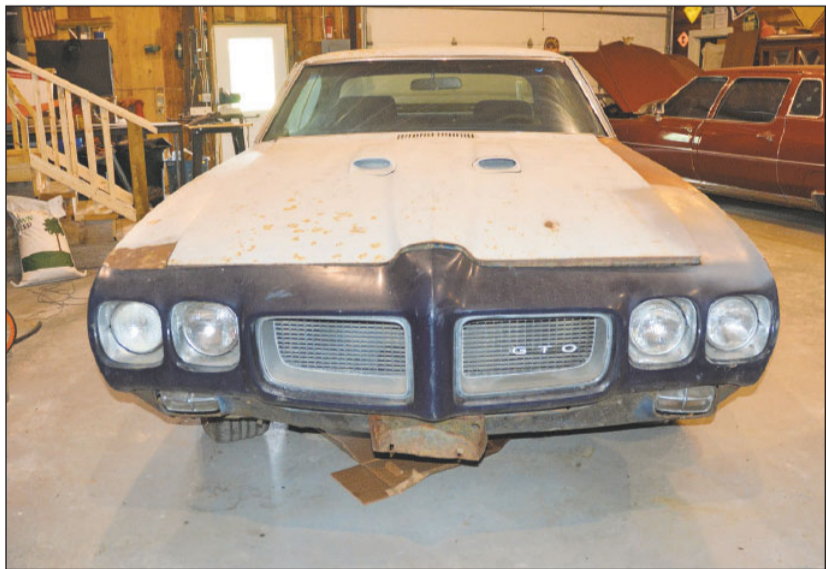
Spotty rust and less than smooth body repairs are features of the GTO that its owner is used to as the car was always a project.
