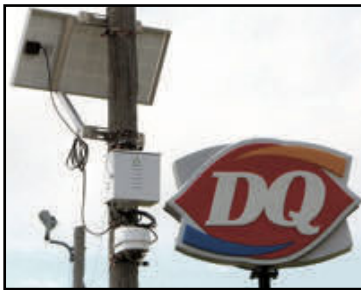
This solar powered camera is recording pedestrian traffic along the highway, as MnDOT gathers data for the scheduled 2024 Highway 108, 59 reconstruction.
