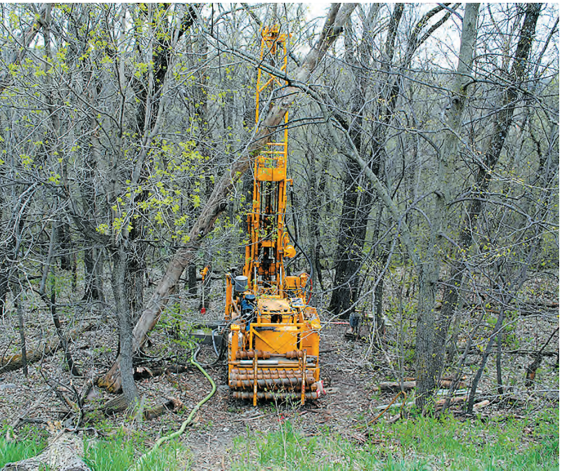
The Minnesota Department of Transportation is in the process of boring electronic sensors into the subsurface at three sites along the shifting earth under state Highway 67 east of the Upper Sioux Agency State Park entrance.
