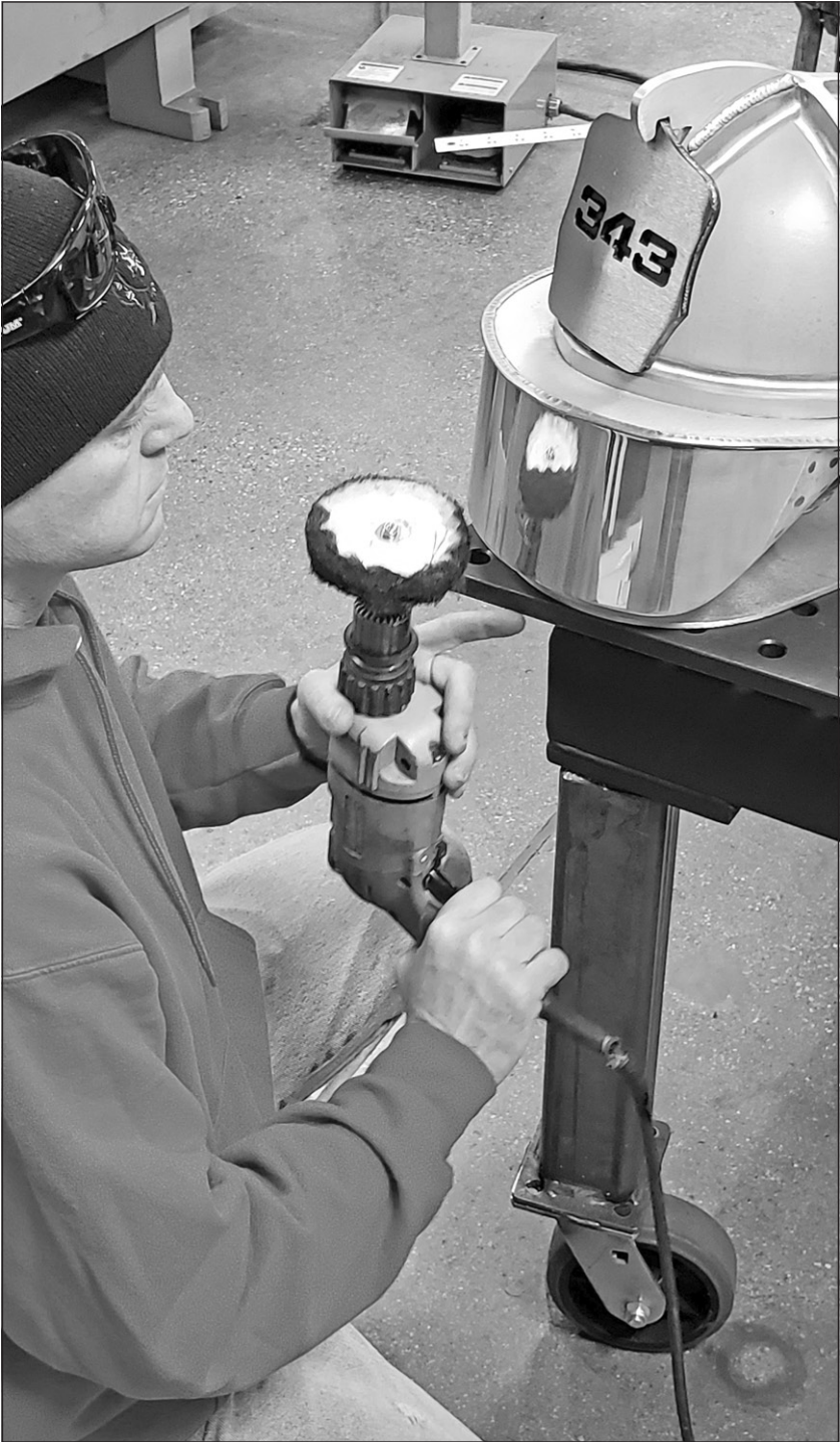
John Travis uses an electric grinder to achieve a mirror-like finish to the shield on his aluminum helmet sculpture.
