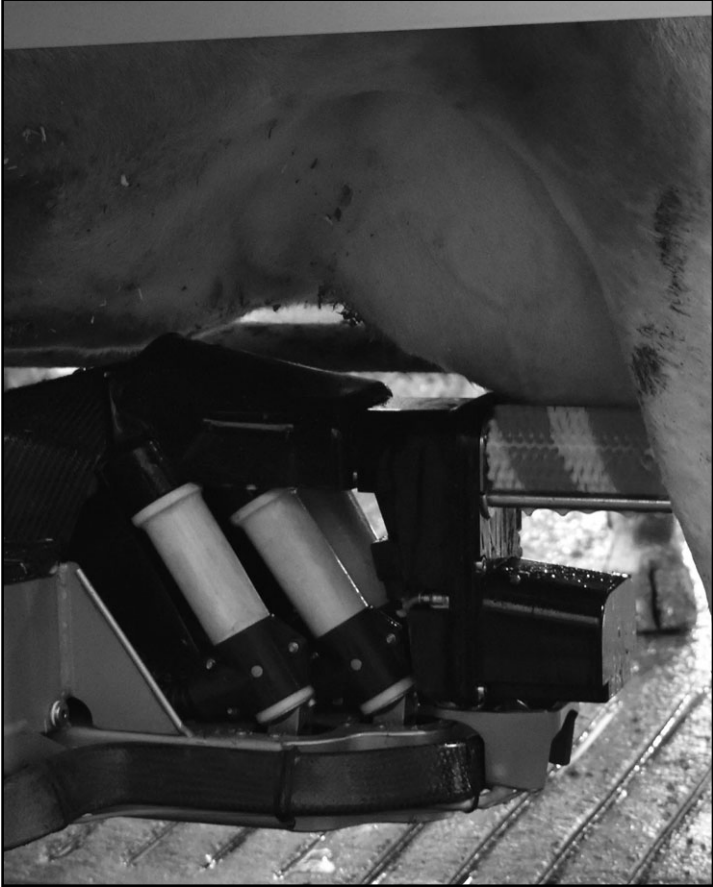
The teats and udder on a jersey dairy cow get washed by a robotic arm with a soft brush before being automatically milked by a Lely Astronaut system the Lingen Dairy Farm invested in.
