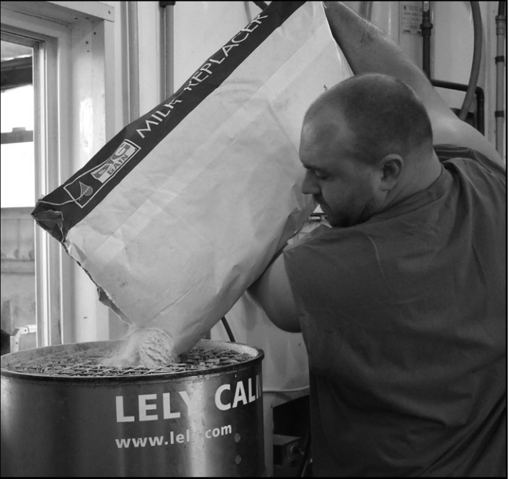
Josh Lingen pours powdered milk replacer into a machine that automatically mixes it with high-quality water and delivers it one at a time to calves, depending on their individual needs.
